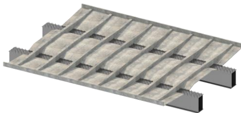
▲ Deck slab elements after being placed on top of the steel girders
